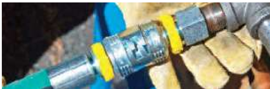
Use Campbell fittings with Nitrogen-Only Warning Rings on the hose and manifold to avoid deadly cross connections
