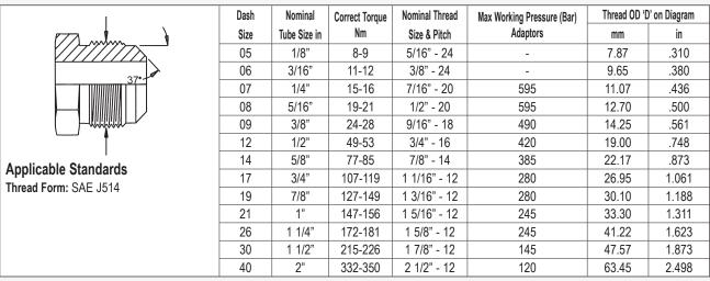
Note: The hex flats from finger tight method is recommended for 37° and 45° flare fittings. The torque values given are for plated carbon steel components without lubrication.
