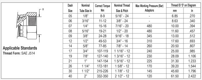
Note: The hex flats from finger tight method is recommended for 37° and 45° flare fittings. The torque values given are for plated carbon steel components without lubrication
