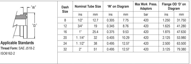
NOTE: Komatsu use flanges that comply with Code 61 and Code 62 in all respects except O-Ring groove dimensions. Refer to Pirtek fittings catalogue Section C for details. They comply to a JIS Standard, and include a Dash 10 size.
