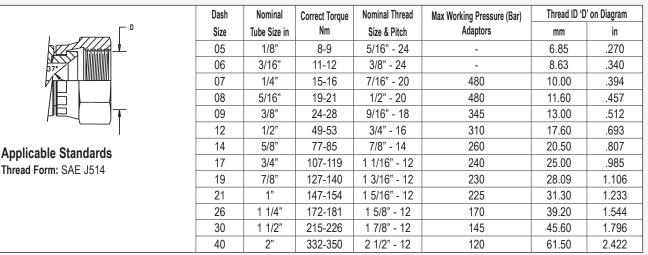
Note: The hex flats from finger tight method is recommended for 37° and 45° flare fittings. The torque values given are for plated carbon steel components without lubrication See page 15
