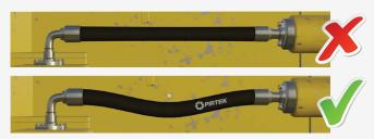
Length may vary +2% to -4% when pressure is applied. Allow enough slack to accommodate this movement. Important to note, that the metal hose fittings are not part of the flexible portion. Allow ample free length for flexing.
