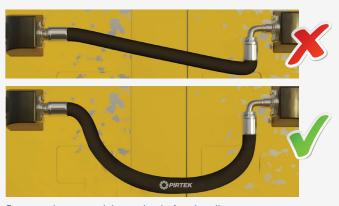
Ensure to have a straight section before bending commences. Using too small a bend radius will greatly reduce flow hose life.
