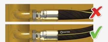
Use the layline to determine that no twist has been induced when tightening. Use 2 spanners to counteract twist.
