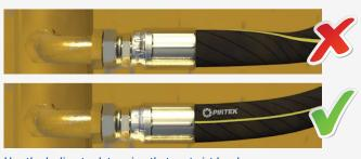
Use the layline to determine that no twist has been induced when tightening. Use 2 spanners to counteract twist.
