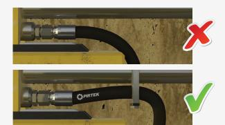
Use clamps to support long runs or keep the hose away from moving parts. Clamps must not be allowed to move as may cause abrasion.
